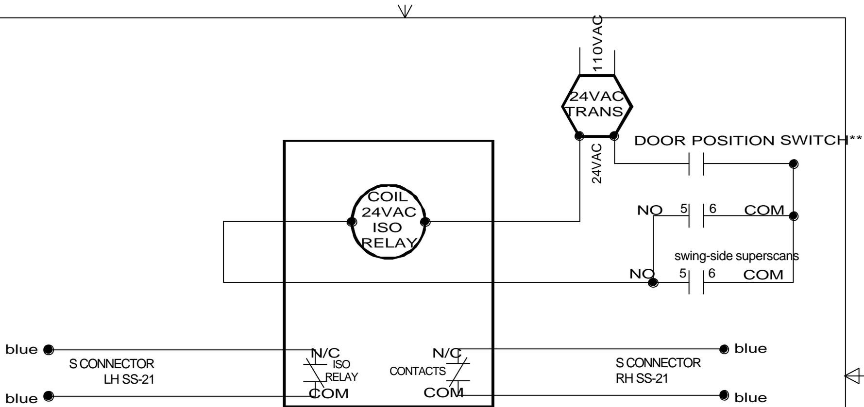
\*\* DOOR POSITION SWITCH MUST BE CLOSED UNTIL DOOR REACHES 70 DEGREES OPEN OR ADJUST TO WHERE DESIRED.
