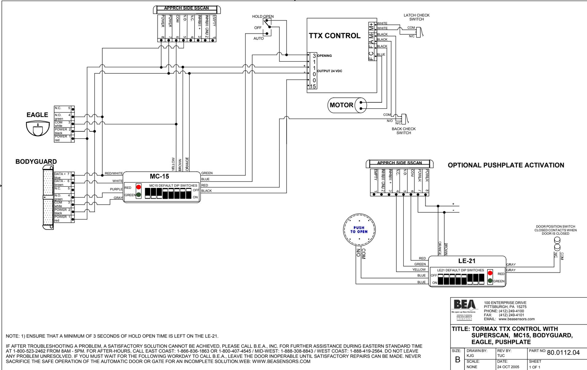
NOTE: 1) ENSURE THAT A MINIMUM OF 3 SECONDS OF HOLD OPEN TIME IS LEFT ON THE LE-21.
