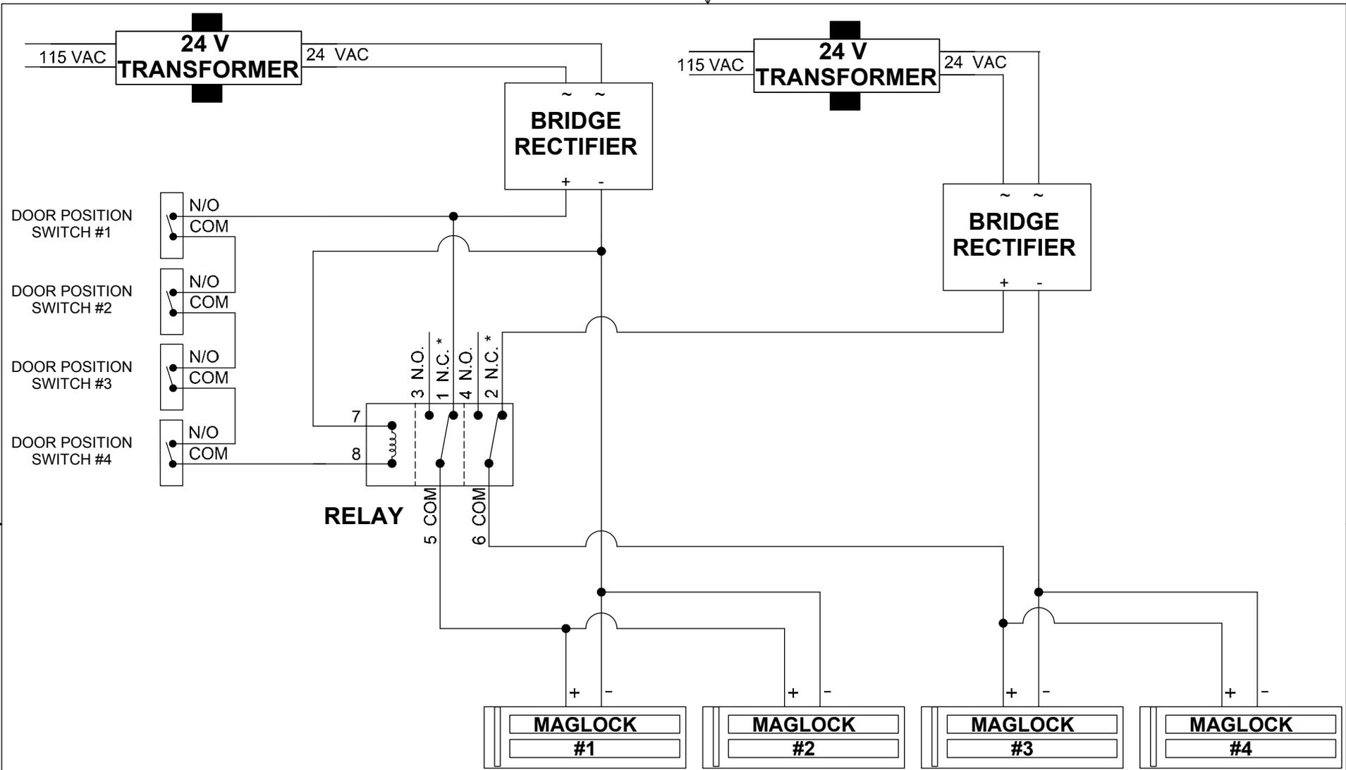
NOTES 1) DOOR POSITION SWITCH CONTACTS MUST BE OPEN WHEN DOOR IS CLOSED. DOOR POSITION SWITCH CONTACTS MUST BE CLOSED WHEN DOOR IS OPEN.
