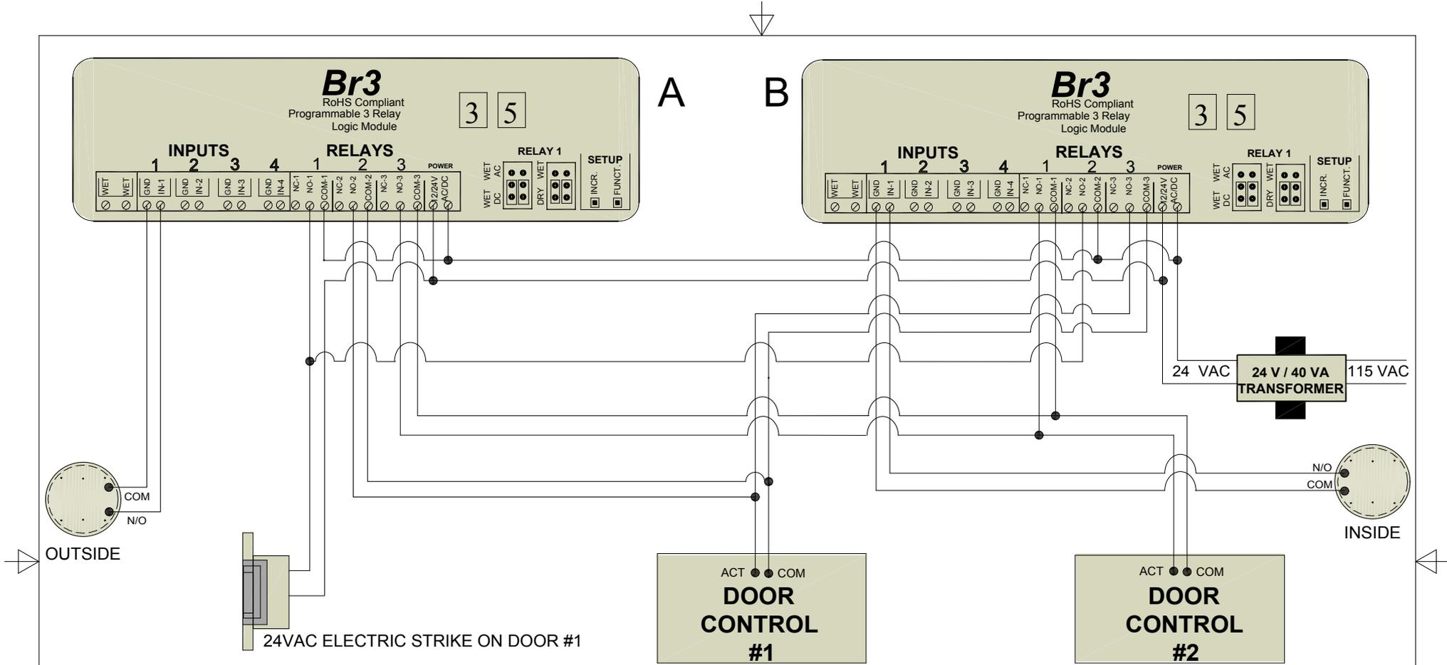
**NOTES:** 1) IF USING AN ACTIVATION DEVICE WITH A WET OUTPUT CONNECT IT TO THE WET INPUT OF THE Br-3.
