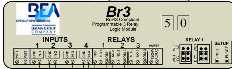
Input 1 and Input 2 are activation inputs for Door 1 and Door 2 respectively
