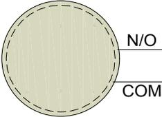
ALL PUSH PLATES WIRE PARALLEL TO IN-1 AND GND
