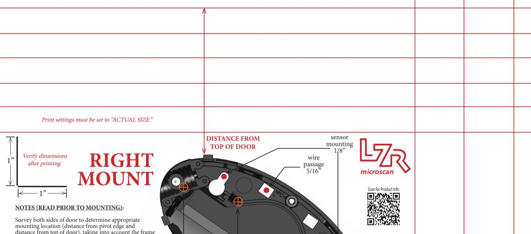
mounting location (distance from pivot edge and distance from top of door), taking into account the frame clearance, finger guard, door arm, etc. Sensors are to be mounted as close to the top of the door and as close to the hinge of the door as possible.
