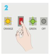
After changing a DIP switch, the orange LED flashes. A long push on the pushbutton confirms the settings.
