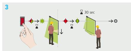
A custom shape can be traced in the whole detection area during the 30-second Learn process. To end this process sooner, push the button again.
