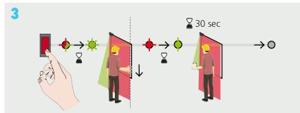
After changing a DIP switch, A custom shape can be traced in the pinch zone during the 30-second Learn process. the orange LED flashes. To end this process sooner, push the button again.
