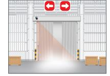
Vertical doors: The best mounting position is left-mount (center-mount is an alternative).
