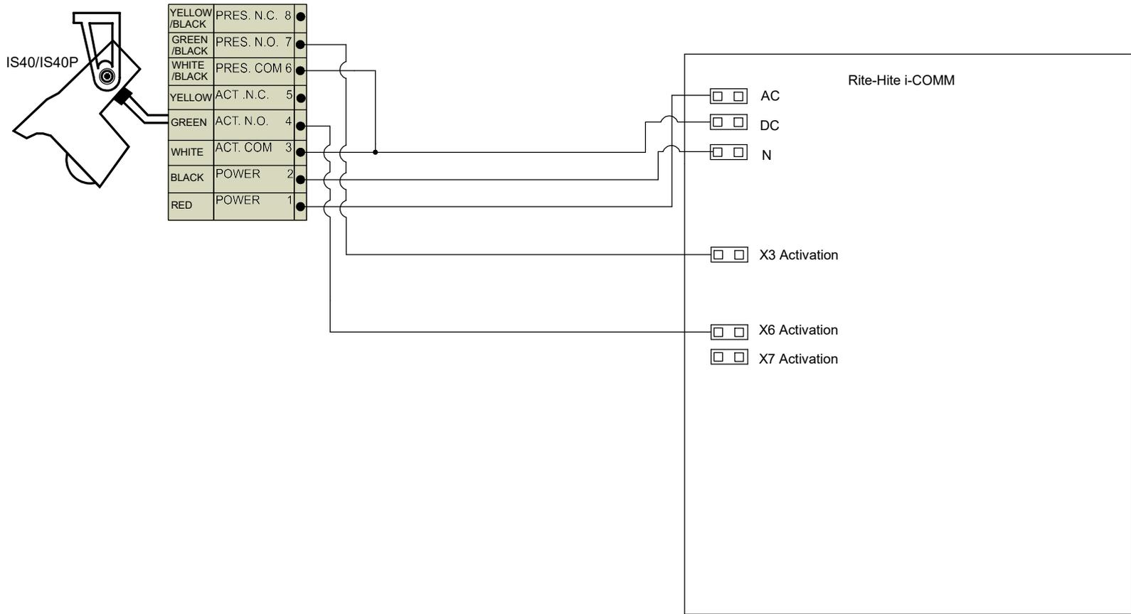
**NOTES:** 1. X3, X6, and X7 are programmable inputs that can usually be used for activation or "reversing edge" type action
